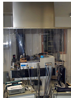
1kHz Ti:SAP Laser: 850nm / 425nm (IR / blue), HighQ Laser and Thales
